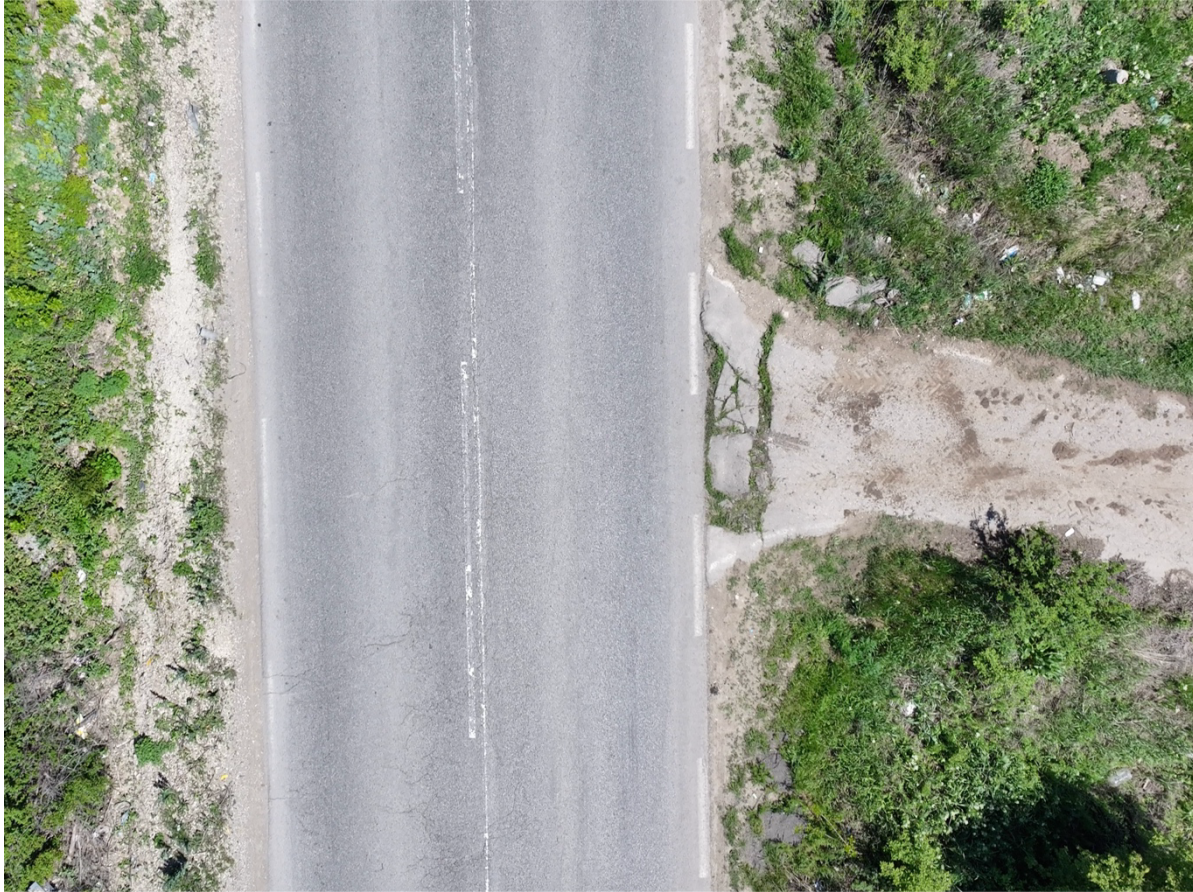
Figure 15 – Unregulated connection at km 65+824. Excerpt from surveying by the remote sensing method in May 2025, performed by the EUCTP team.
